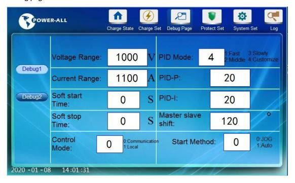
Debug1: Charger debug interface, these default parameters have been pre-set at factory before shipment, end user is no need to modify
