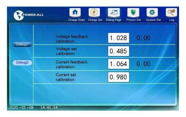
Debug2: Calibrate voltage and current in the debug interface. If recalibration is needed, please do not change too much, just a little. For example, 1.028 change to 1.030, not to 1.30.
